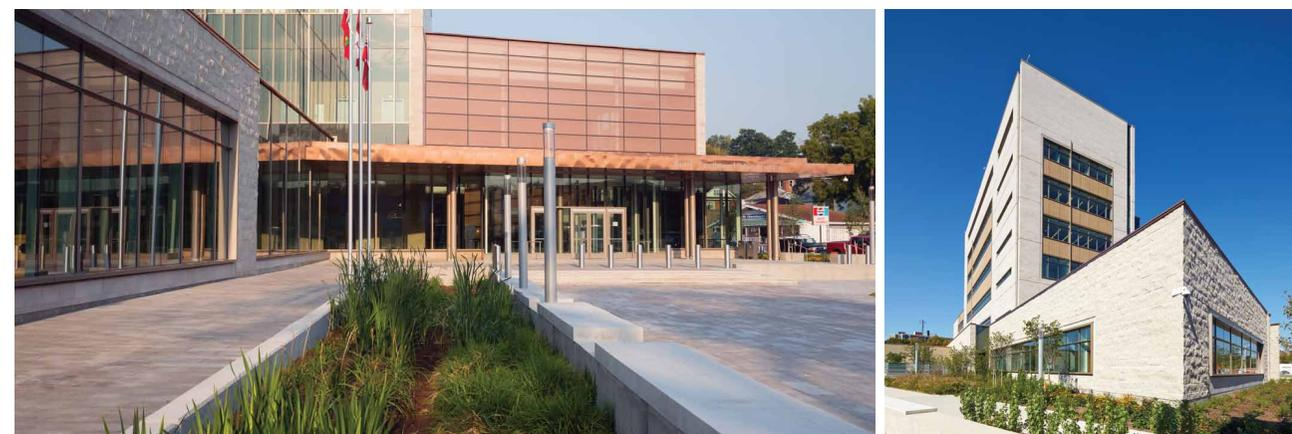
The courthouse's appearance and character have been designed to transform, as time passes: the contemplative garden wall is topped with copper, which will eventually oxidize and turn green; the copper of the main entrance's canopy will age the same way.
